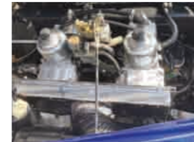
Original fabricated plenum air box
