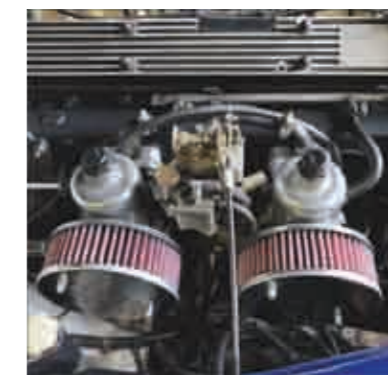
Newly fitted K&N air filters
